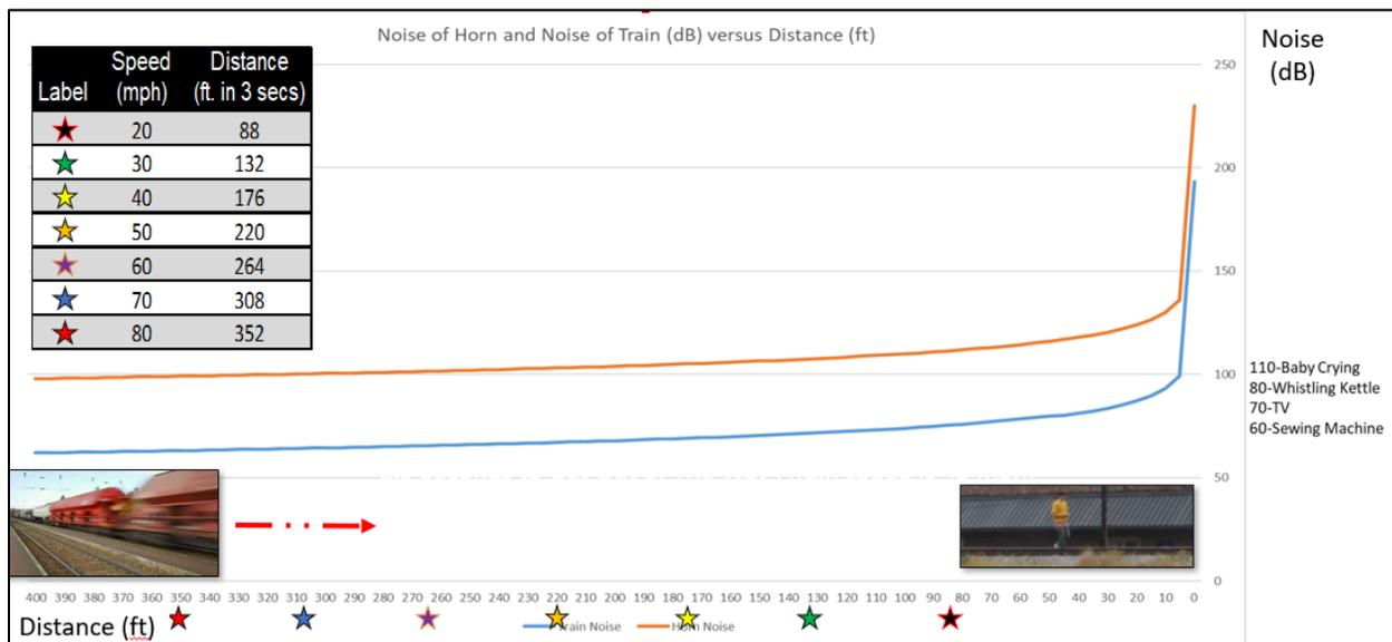
Figure 6. Train horn noise in space and time while considering perception and reaction time and speed of train
