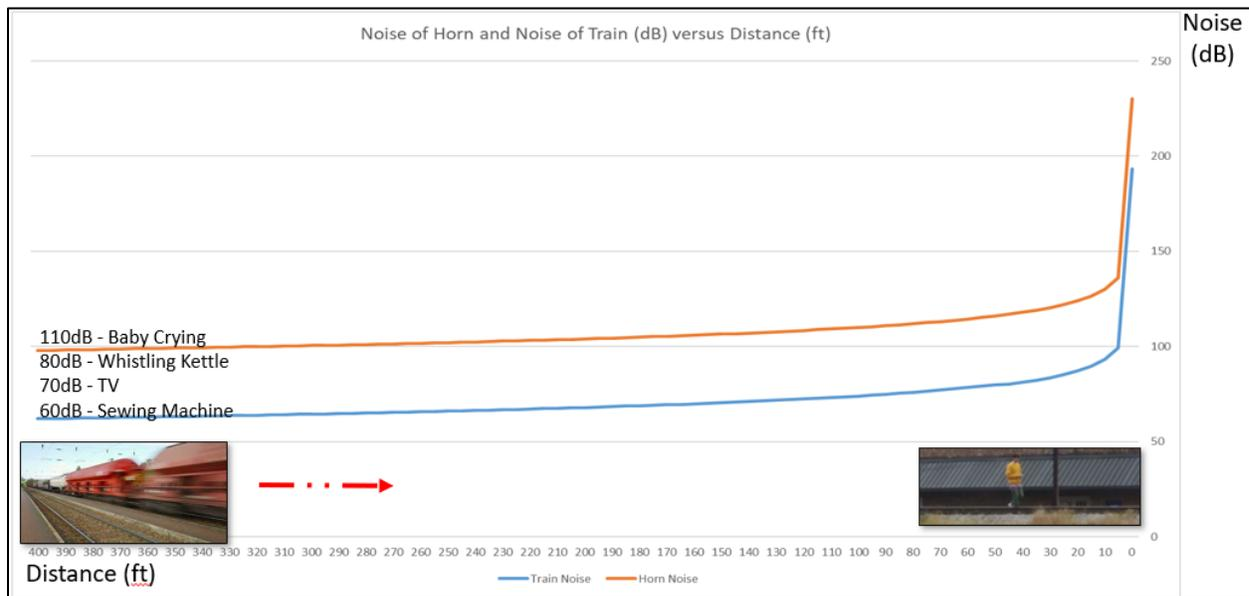
Figure 5. Train horn noise in space and time compared to everyday noises
